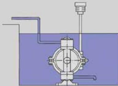
Lutz-JESCO double diaphragm pumps can also be operated when submerged. Care should be taken with respect to the materials in contact with the liquid. Also, the air outlet needs to be above the liquid level.
