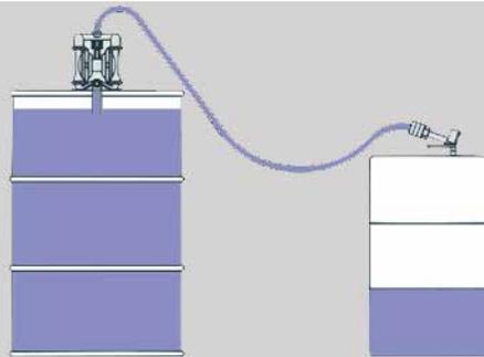
Lutz-JESCO's double diaphragm pumps are also ideally suited when pumping abrasive, dense and/or highly viscous liquids from drums and containers. To facilitate these applications, the 1/2" and 1" sizes can be supplied with suction pipe and adapter.
