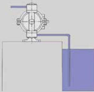
When the suction of the pump is above the level of the liquid, the pump has to prime the medium. In dry conditions, the Lutz-JESCO double diaphragm pumps have a lift capacity of up to 14.8 ft.
