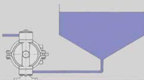
When the liquid level is above the suction of the pump, the pump suction is considered positive or flooded. Under this condition the intake can be regulated by a suitably sized valve.
