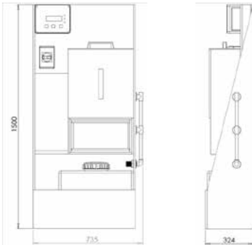
Fig. 7: Dimensions EASYCHLORGEN Compact SKID-1
