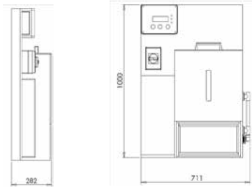
Fig. 6: Dimensions EASYCHLORGEN Compact Modular
