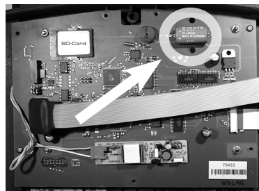
Fig.9: Battery for internal clock, on the display circuit board.
