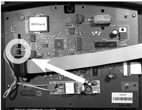
Fig. 6: Cable connections for protected cable passage to the rear part of the housing.
