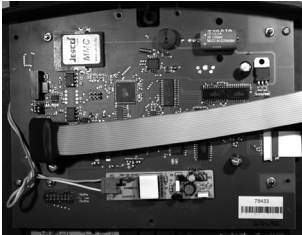
Fig. 41: Slot for the memory card on the display board. The card is inserted on the display circuit board in the front housing.
