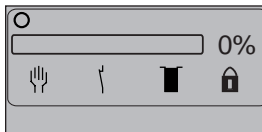
Fig. 26: Start screen with activated password protection
