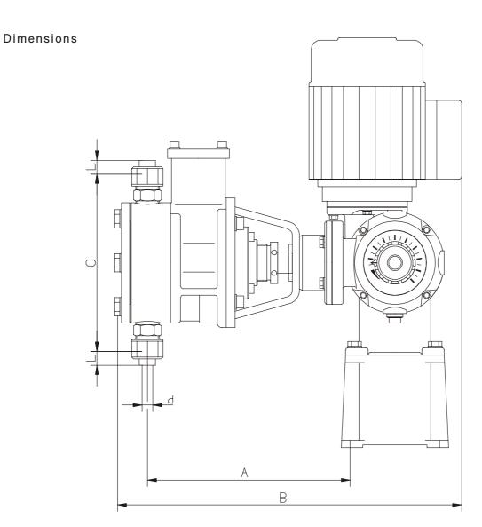
For dimensions L and d, see Table 5 (connections) of the relevant pump data sheet. The pump dimensions can be found in the data sheets as well.
